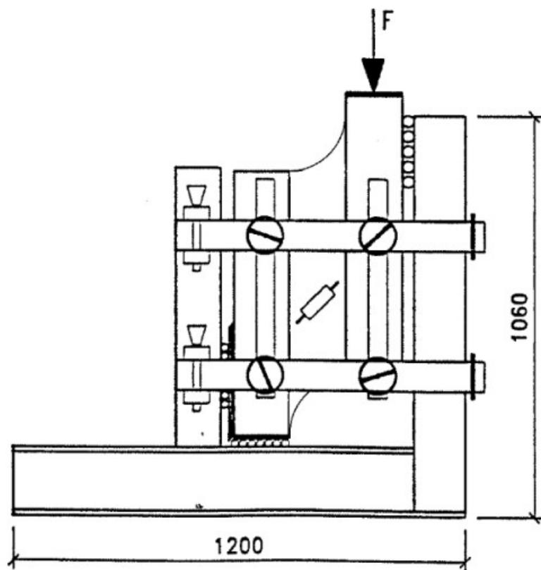
Figure 6 - Loading arrangement for panel shear test
