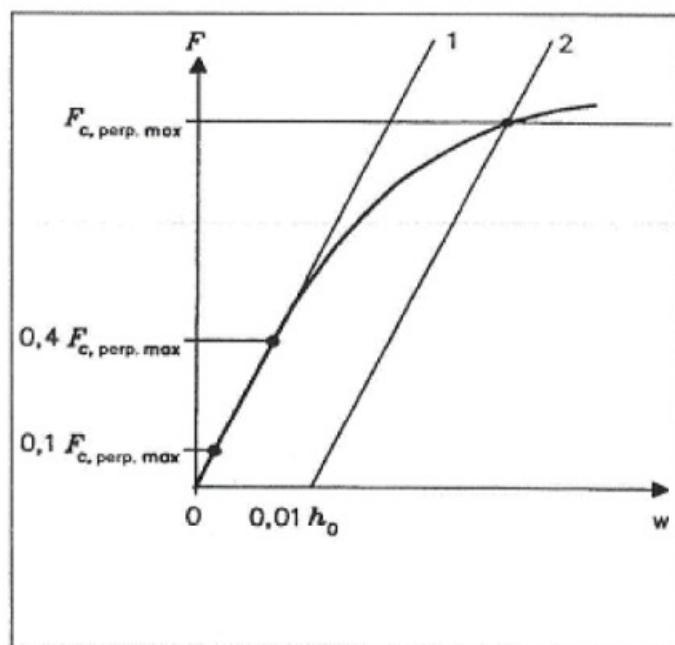
Figure D.2 – Load – deformation diagram for the compression test perpendicular to the plane of the panel
