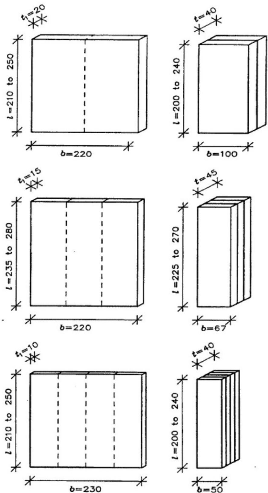
Figure A.2 - Examples of test pieces from panels having a thickness of less than 40 mm
