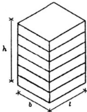
Figure D.1 – Composite glued test piece for compression test perpendicular to the plane comprising a number of identical layers
